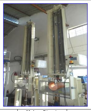
18. Vibration Leakage Tester
