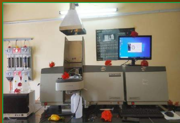
Atomic Absorption Spectroscopy (AAS) machine installed at Mysuru centre on 3 rd April, 2023.
