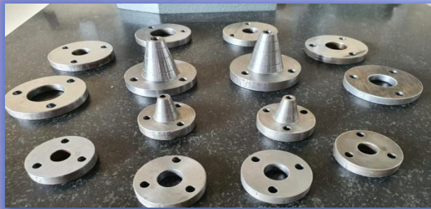
Cone type End fitting & fixtures developed for Hydrostatic Pressure Testing of Plastic Pipes
