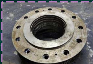
Machining of Hydraulic Flange in CNC VMC.
