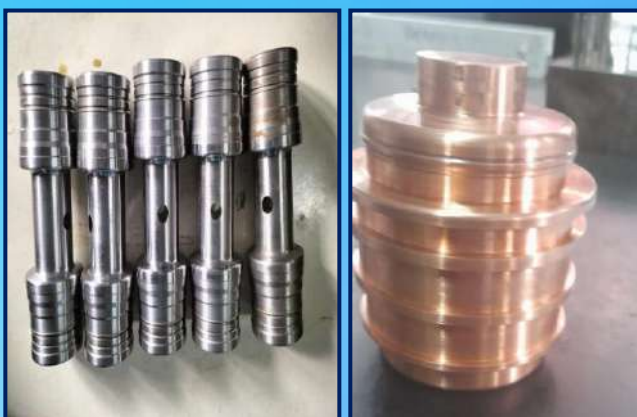
Product Name: Machining of Core Insert and Electrode for Rubber Mould. Centre: Chennai
