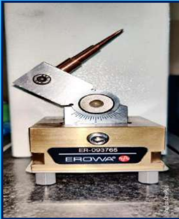
Product Name: Developed degree Electrode Holder of EDM Machine for Machining Sub-Surface gating in Injection Moulds Centre: Murthal
