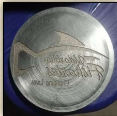
Product Name: Logo Embossing on Steel plate using CNC EDM Machining Centre: Bhopal
