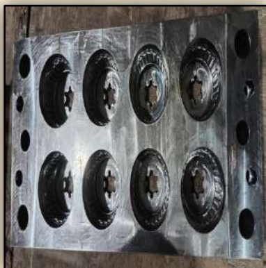
Product Name: 8 Cavity Die Set for Clay Katori/Bowl Centre: Bhopal
