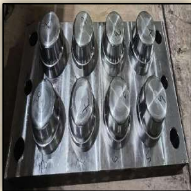
Product Name: 8 Cavity Die Set for Clay Katori/Bowl Centre: Bhopal
